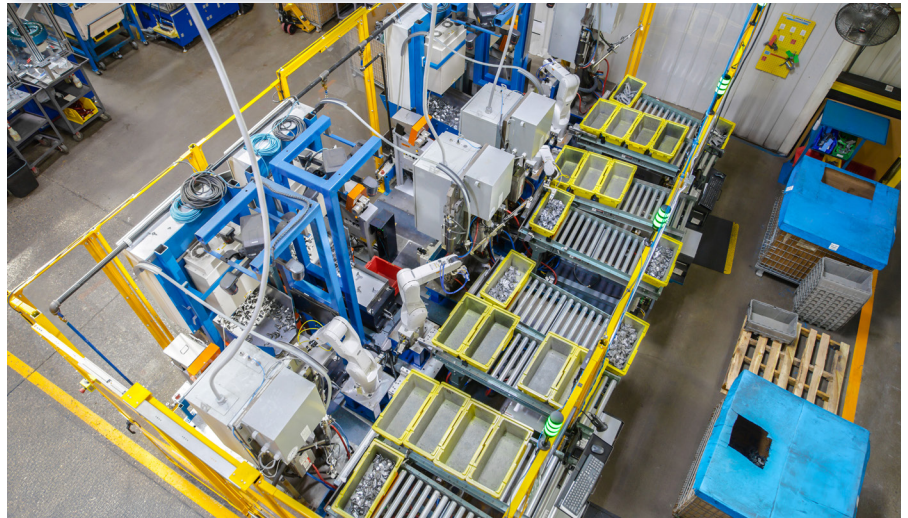
4 Robot nut welding cell developed by BTD's Corporate Automation team. It uses computerized vision cameras to communicate part orientation to the robot, so parts have no need to be staged.
