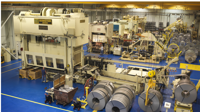
One of BTD's 3 Stamping rooms. This one features 600 - 1,200 ton presses
